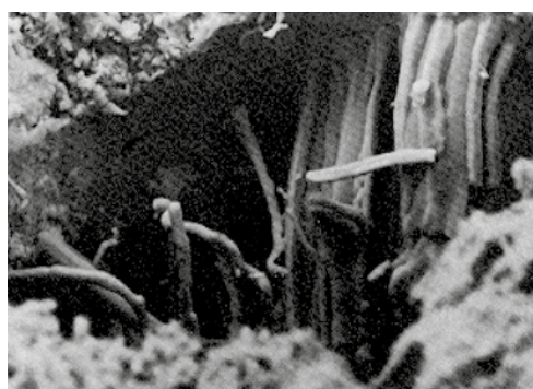
The cristallization of the salts in the pores of the KÖSTER Restoration Plaster prevents the salts to cause damage.
